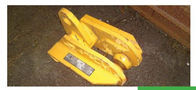
he Thomson Engineering Drag Clamp has a unique cam action rail gripping system which tightens its grip on the rail the harder you pull.
